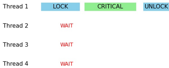
Figure 1: Contention and Blocking: Only one thread can access the critical section at a time. Others must wait.
